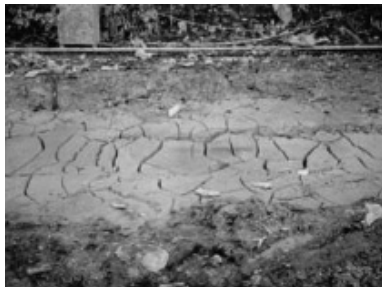
Bentonite for Impermeable Wall
