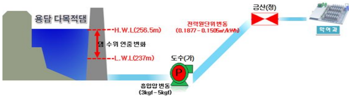
[Figure 4-7] Changes in pump operation curves
