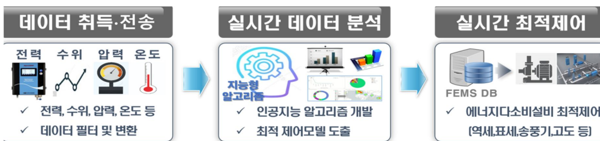
[Figure 4-4] Principles of AI-based EMS construction
